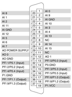
NC = No Connect NI PCI/PXI-6233 Pinout
