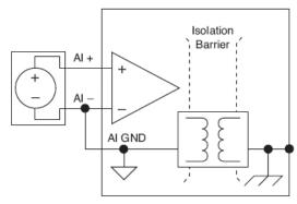
Figure 1. Isolation Barrier on Industrial M Series Devices
