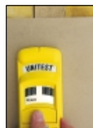
Detects wood i.e. roof battens
